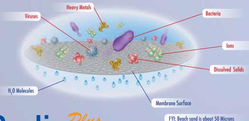
Water pressure forces smaller  $H_20$  molecules through very tiny semi-permeable membrane pores, which measure 0.0001 microns. This acts as a barrier to contaminants, which are rejected by the membrane and flushed down the drain.
